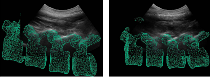
Fig. 5. Examples of the registration. The multi-vertebrae model is capable of capturing different sizes, shapes and poses of vertebrae.
