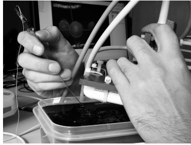
Fig. 4. Navigated US-guided needle insertion into a gel phantom. Note the needle and the field generator directly above its entry point.
