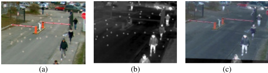
Fig. 2. An example of image fusion: (a) video camera image, (b) thermal camera image, (c) aligned images. White circles show the positions of fusion points.
