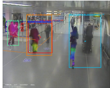
Fig. 6. Sample events detection results. Left column: video frames illustrating the event, right column: visualization of the algorithm, where orange lines denote barriers, multi-colored rectangles – object trackers and multi-colored semi-transparent layers – velocities of objects exceeding minimum speed threshold (different directions of movement are represented with different hues while velocity vector magnitude is directly proportional to the layer luminance)
