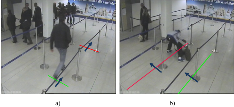
Fig. 3. Example of input (green) and output (red) barrier placement for the counterflow (a) and border crossing (b) events detection; dark arrows denote direction of movements associated with barriers
