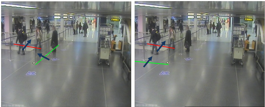
Fig. 5. Example of input (green) and output (red) barrier placement for the two variants of the border crossing event; dark arrows denote direction of movements associated with barriers
