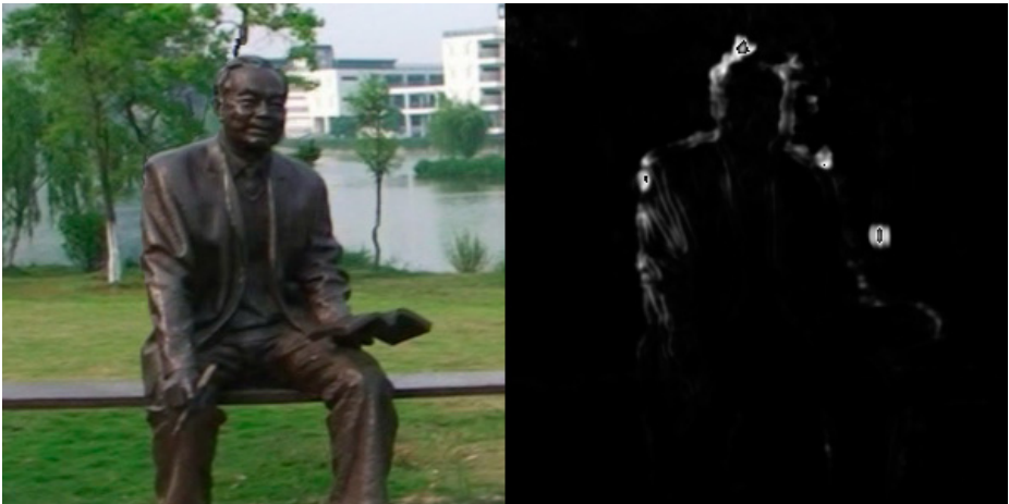
Fig. 10. Fragments of synthesized view and SSIM metric visualization for 16th frame of the “Statue” sequence with constant key frames distribution. On the metric visualization lighter areas correspond to lower metric values. SSIM = 0.993088 .
