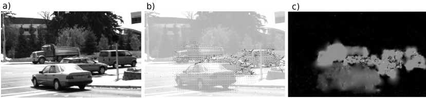
Fig. 1. Optical flow estimation: (a) one frame from a sequence; (b) displacement vectors; (c) flow visualization. Image sequence from Middlebury dataset [6].
