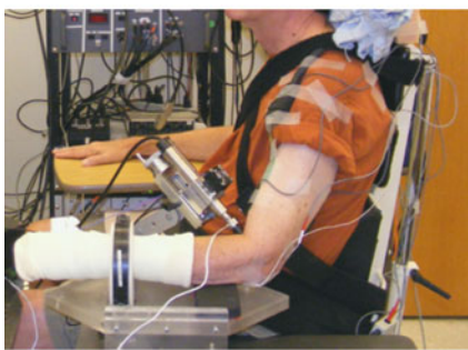
Fig. 7.3 A device for automatized tendon tapping measure. Left experimental set up: a position-controlled linear actuator (Linmot, Inc.) is placed perpendicular to the tendon of the biceps brachii, while the tension in the stimulated muscle tendon and the EMG activity of that muscle are measured; Right exemplary force trace recorded by the force sensor during tapping (Chardon et al. 2009)
