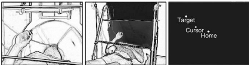
Fig. 5.2 Center-out hand movement adaptation set-up. In the left and middle panels , a subject is shown lying with his head inside the MEG recording dewar holding an optic pen on a sheet of glass. Note that vision of the hand and upper limbs is occluded with a black cloth . The right panel depicts the subject's view of the computer screen where visual feedback of the pen position ( cursor ), center location ( home ), and peripheral target ( target ) was displayed in real time. From Bradberry et al. (2009), with permission
