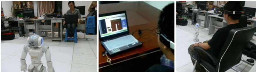
Fig. 79.4 Motor imaginary based humanoid robot navigation control in experiment
