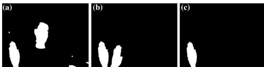
Fig. 12.7 Hand region extraction (2) a skin color detect result (2), b motion mask result, c hand segmentation result (2)
