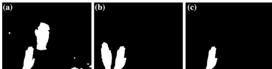
Fig. 12.6 Hand region extraction (1) a skin color detect result (1), b motion mask result, c hand segmentation result (1)
