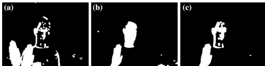
Fig. 12.3 Skin color mask (1) a motion detection result, b skin detection result (1), c mask result (1)
