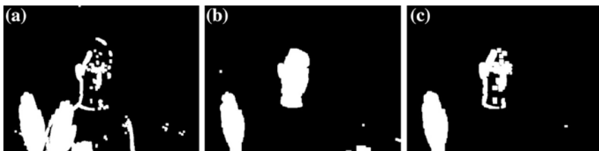
Fig. 12.4 Skin color mask (2) a motion detection result, b skin detection result (2) c mask result (2)
