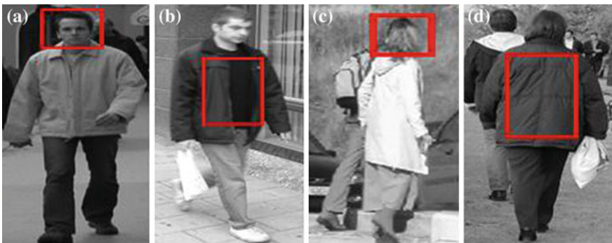
Fig. 46.2 Part of the experimental effect diagram. a, b Shows respectively detecting no-occluded pedestrians with a single head and torso detector, which can accurately detect people; and c, d shows respectively detecting occluded pedestrians with the same detector, which will cause undetected
