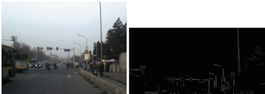
Fig. 69.6 The results obtained from the LCP operation. Left is the original image, right is the results obtained from the LCP operation
