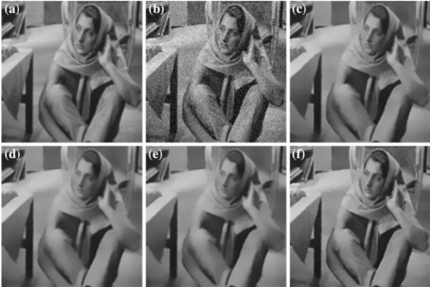
Fig. 88.1 Image denoising results based on different algorithms: a Original image; b noisy image; c method in [11] with h = 1.2\sigma ; d method in [11] with h = 1.4\sigma ; e method in [1] h^2 = 10\sigma , 2007; f our method
