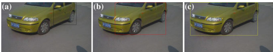
Fig. 45.2 Nonlinear object tracking result from different tracking method. The EKF algorithms use black box, The UKF algorithms use red box. Our NMKF algorithms use yellow box. a EKF. b UKF. c NMKF
