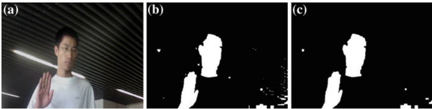
Fig. 12.1 Skin segmentation a original image, b result of skin segmentation, c corrosion and expansion results
