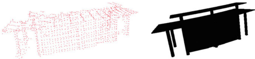
Fig. 1.2 The relationship between point cloud model and VRML model, left point cloud; right VRML model
