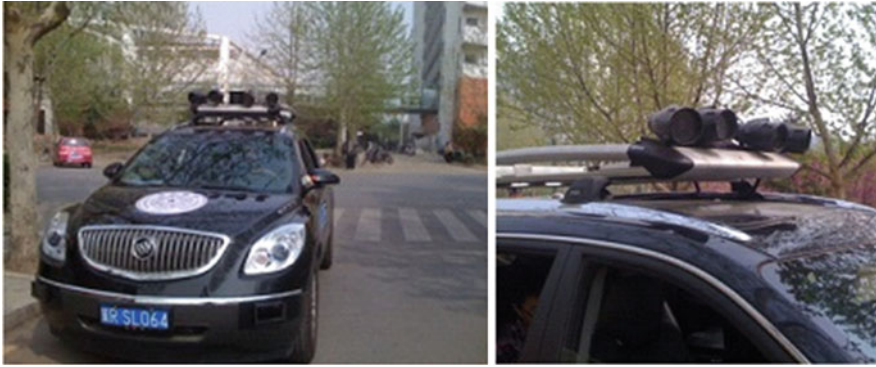
Fig. 69.3 The experimental platform. Left is THU-ALV2, right is the color camera installed
