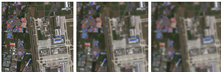
Fig. 36.1 From left to right : original image, original image blurred with an averaging filter, blurred image re-blurred with the same averaging filter
