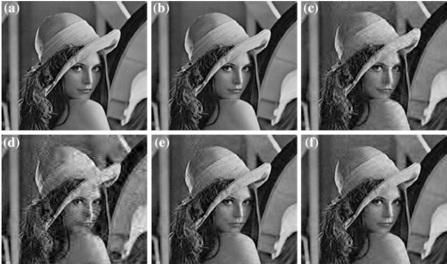
Fig. 89.1 Comparing results between algorithm based on Wavelet and NSCT, (a) is original image, (b), (c) and (d) are reconstructed image based on Wavelet when M = 200, 150, 100 respectively. (e) and (f) are reconstructed image based on NSCT when M = 100, 50 respectively
