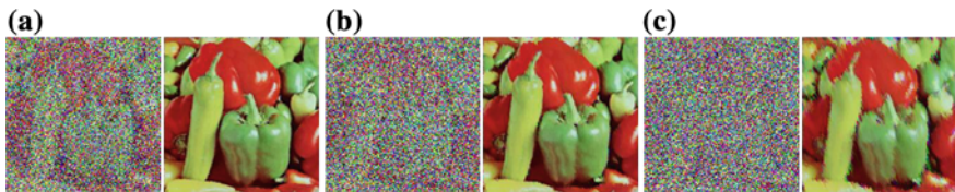
Fig. 41.5 Corrupted and denoised images of “peppers” at different highly noise densities. a 70 % noise density. b 80 % noise density. c 90 % noise density
