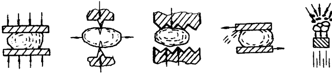
Fig. 75.1 Several roles in the form of broken coal machinery to material. 1. Squeezing; 2. Split; 3. Fracture; 4. Mill; 5. Shredding
