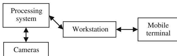
Fig. 31.4 Schematic diagram of mobile terminal monitoring
