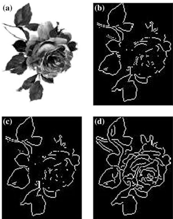
Fig. 182.1 The edge-detection results for different method. a original image, b sobel operator, c prewitt operator, d canny operator
