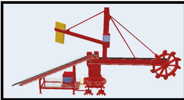
Fig. 157.2 Stacker and reclaimer
