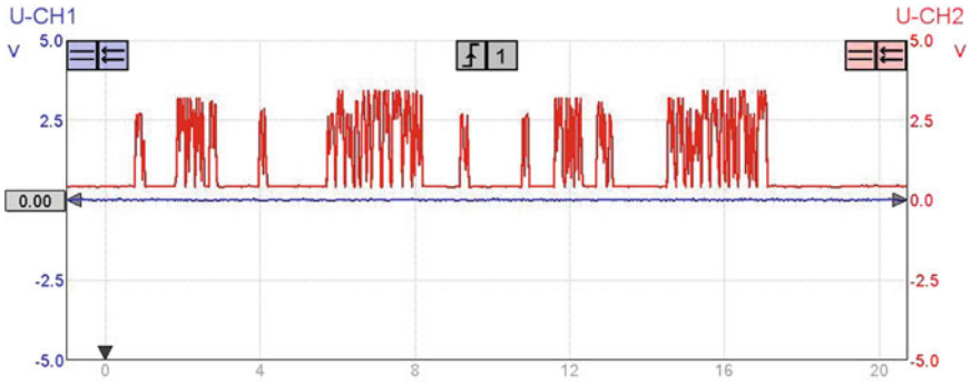
Fig. 29.6 CAN_L short circuit to negative electrode
