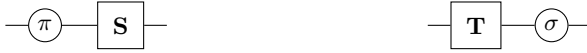
Fig. 1. The real (left) and the ideal (right) setting considered for reducibility in the context of indifferenciability
