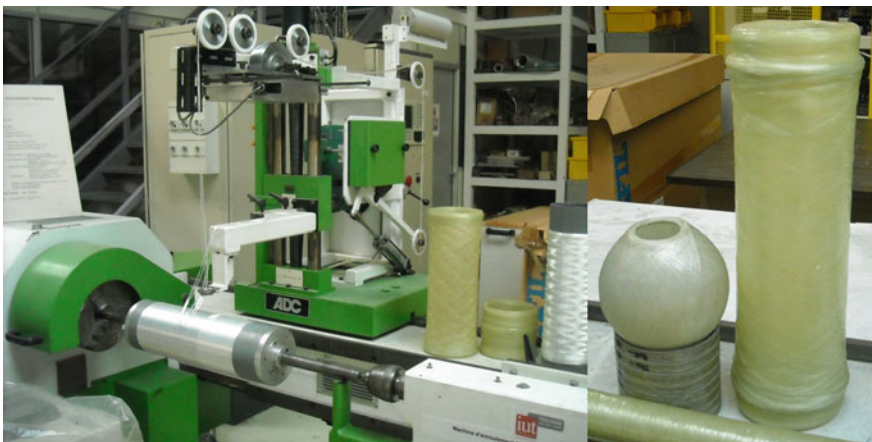
Fig. 1.2 Filament winding process (UPS, Toulouse)
