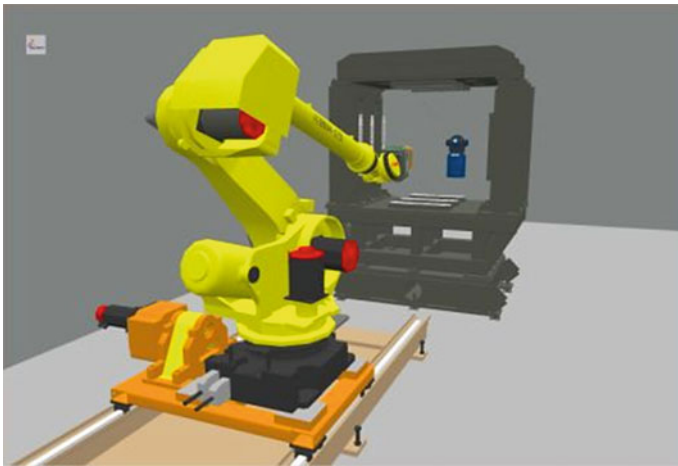
Fig. 1.6 System used for drilling fuselage in aerospace industries ( www.sae.org )
