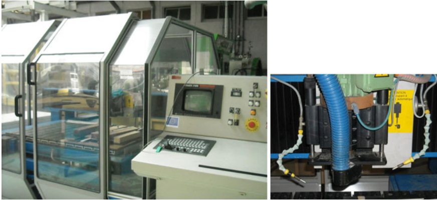
Fig. 1.5 CNC machine used for machining composites with vacuum system (UPS, Toulouse)
