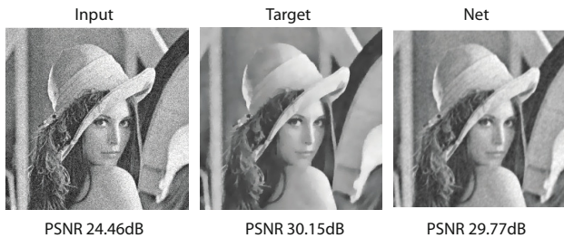
Fig. 8. Total Variation (TV) task. The network has to learn to approximate the TV output (target) by means of averaging two filtering pipelines.
