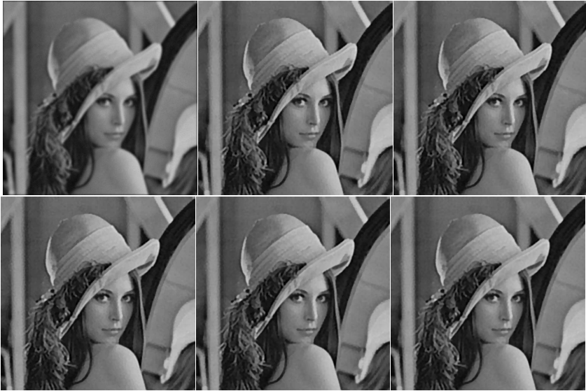
Fig. 4. Illustrates results of deblurring technique with various regularization methods. Top row: noisy and blurred input image, TV regularization [3] and BTV regularization [8]. Bottom row: deblurred image using geodesic regularization, Morphologic regularization [4], and Adaptive morphologic method. (Quantitative comparisons are in text).
