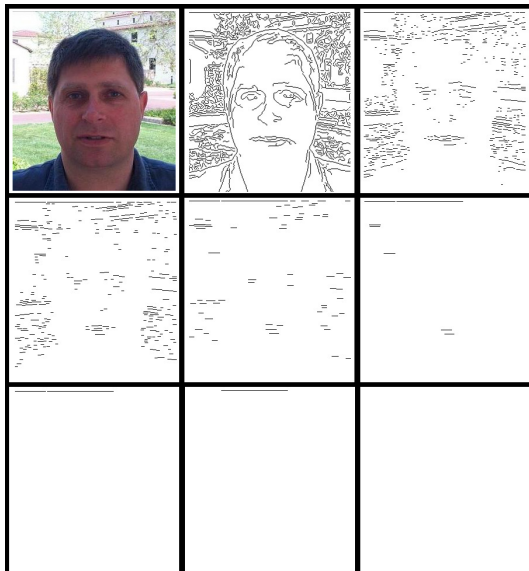
Fig. 1. Steps to compute the pattern spectrum for an image of class Faces_easy. The family of SEs used has 0° of orientation. From top to bottom, left to right, the images are: original image, map of edges, results of morphological opening using a linear SE with 2, 4, 8, 16, 32, 64 and 128 pixels of length, respectively.
