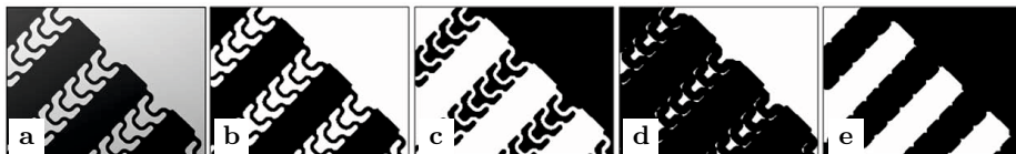
Fig. 2. The results of the intermediate steps of calculating the mean channel depth. Left to right: (a) Raw image – (b) Segmentation of upper surface – (c) Segmentation of channel layer – (d) Erosion of (b) – (e) Erosion of (c).
