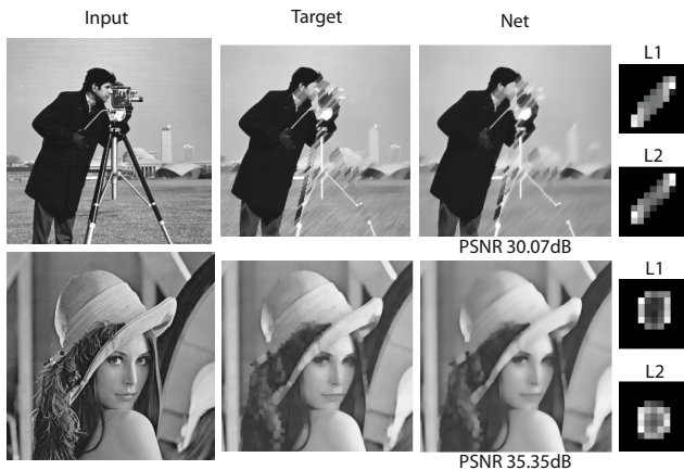
Fig. 4. Top: an example of learning a closing operator where a line of length 10 and orientation 45^\circ is used. Bottom: opening with a square structuring element of size 5. The network closely matches the output and almost perfectly learns the structuring elements in both PConv layers.
