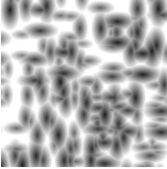
Fig. 4. Example of simulation of a Boolean random function with elliptical cones in two orthogonal directions. The primary functions start from different values (image 256 x 256).
