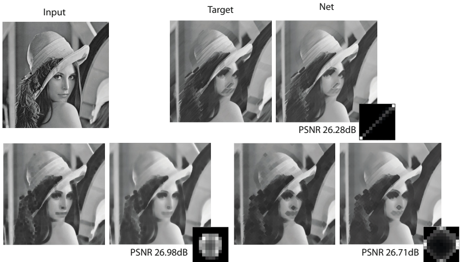
Fig. 3. Examples of learning an erosion with three different structuring elements along with the learned kernel w(x)
