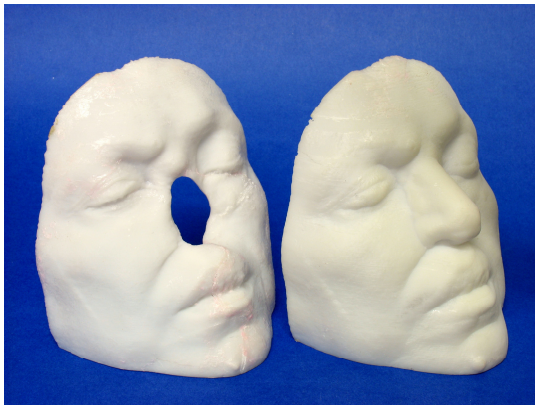
Fig. 13. Physical copies obtained by means of SLA machining
