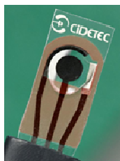
Fig. 1. A screen-printed three-electrode system. (1) working electrode; (2) reference electrode; (3) counter-electrode.
