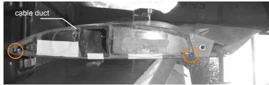
(a) Sensors S1 and S2 of measurement set 1 at the left wing, laying in the connection wing-winglet. The electrical cables pass through a small duct leading to the cockpit;
