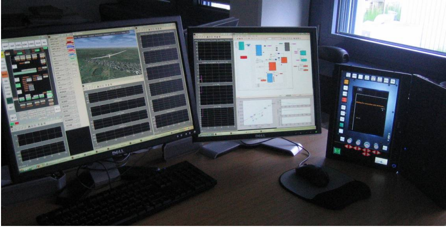
Fig. 2 Work station and Automatic Flight Control Panel (AFCP) for flight control law development
