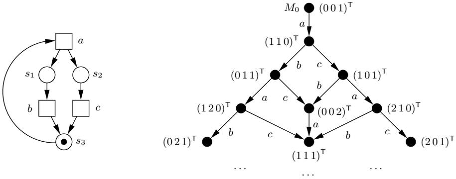
**Fig. 6.** Neglecting the token: structurally live, but not structurally bounded
