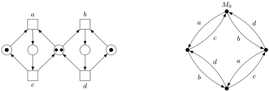
**Fig. 29.** A net which is persistent and BiCF but not BCF (l.h.s.), and its reachability graph (r.h.s.)
