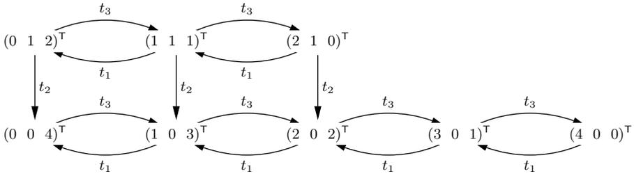
**Fig. 3.** The reachability graph of the Petri net shown in Figure 2; the initial marking is  $(0\ 1\ 2)^T$
