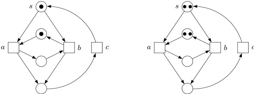
**Fig. 33.** A persistent Petri net (l.h.s.) and its non-persistent 2-multiple (r.h.s.)
