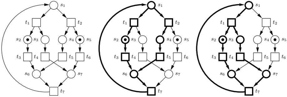
**Fig. 21.** An initially marked FC-net (l.h.s.); an S-component (middle); a T-component (r.h.s.)
