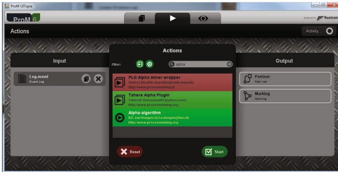
Fig. 34. ProM 6 Action Browser; selecting the alpha -miner to discover a process model from the loaded event log
