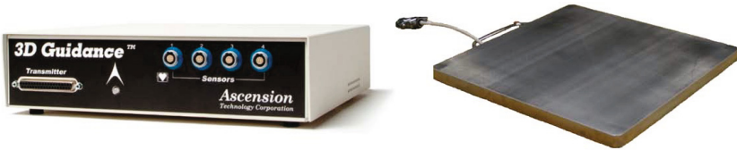
Fig. 3. The EM tracking system that was used here includes the control unit ( left ) and the fat-type magnetic field generator ( right )
