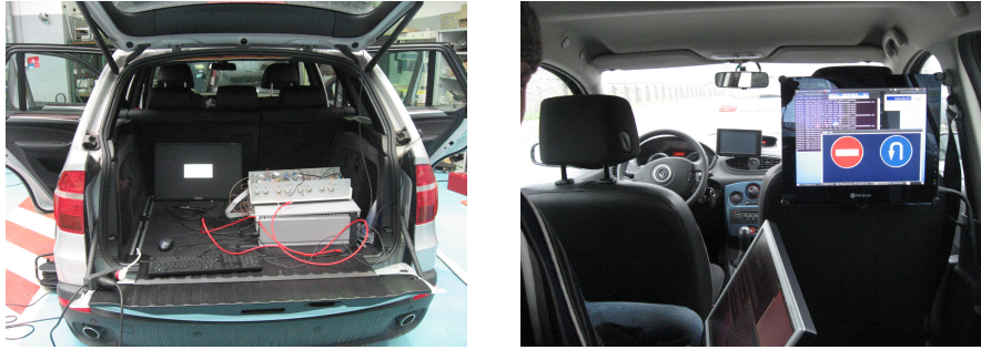
(a) Integration of the SDR platform on a BMW X5 test vehicle
