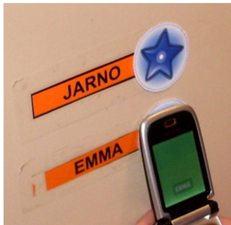
Fig. 2. A nametag “JARNO” equipped with an NFC tag and a star icon. The tag is placed behind the star icon.
