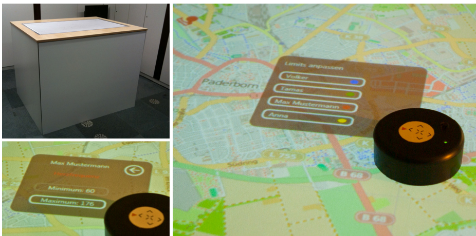
Fig. 4. Picture of the useTable (top left) and a tangible object allowing an authenticated changing of heart rate limits (right: select patient, bottom left: change limits)
