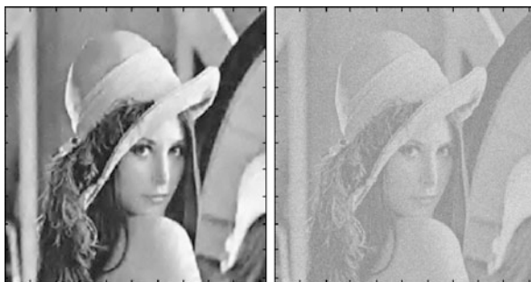
Fig. 13.13 Right: Noisy Lena image (Noise is white and Gaussian with \sigma = 35 ) and PSNR = 17 dB. Left: Denoised Lena using 4-level-sigmoidal wavelet shrinkage, PSNR output = 30 dB
