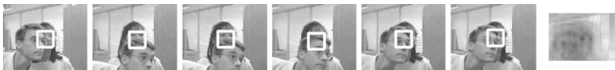
Fig. 4.1 PSO based tracking using multi-patch object representation. Frames #431, 441, 453, 455, 460, 461, and the probability image of the target in frame #431
