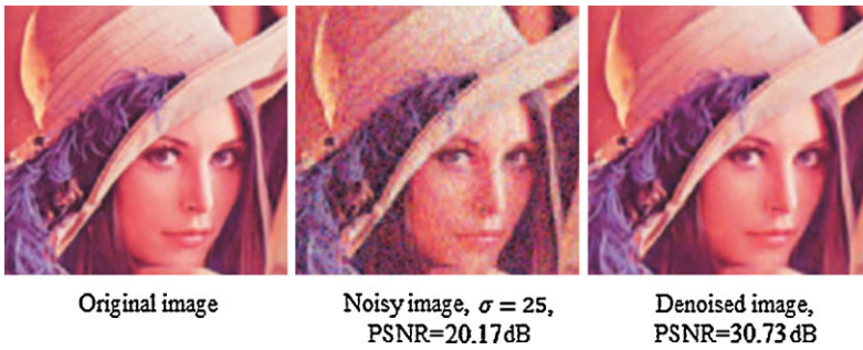
Fig. 13.14 Denoising based on estimation of the probability of the presence of useful information: 3-band Lena (RGB)
