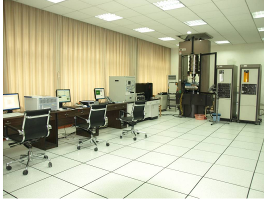
Fig. 1 MTS815 Flex Text GT rock mechanics test system
