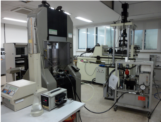
Fig. 2 View of experimental set-up of multistage triaxial compression test under elevated temperature condition
