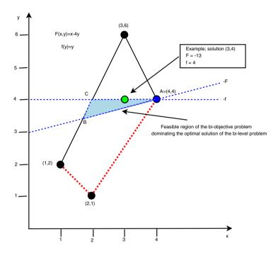
Fig. 1.2 Bi-level optimization versus bi-objective optimization (2)
