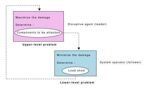
Fig. 1.3 Vulnerability analysis of the electric grid under terrorist threat
