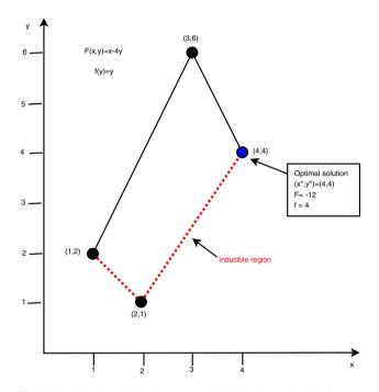
Fig. 1.1 Bi-level optimization versus bi-objective optimization (1)
