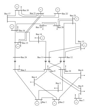
Fig. 2.7 IEEE One Area Reliability Test System
