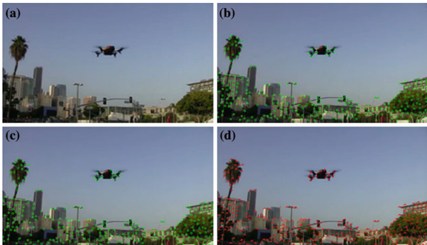
Fig. 2 a out door environment b features detected on image It c features detected on image It+5 d optical flows between the two images
