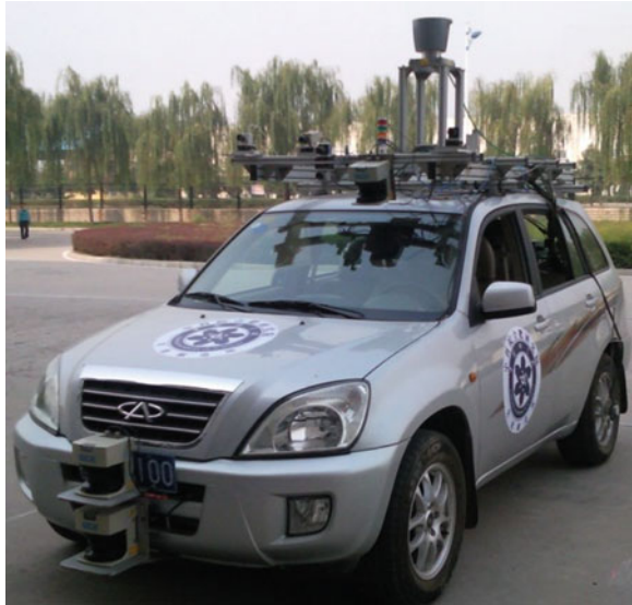
Fig. 7 Intelligent pioneer with cameras mounted on top of the vehicle
