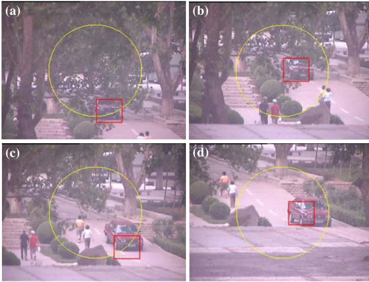
Fig. 5 An example of tracking a vehicle using a PTZ camera. a Frame 7. b Frame 129. c Frame 459. d Frame 507
