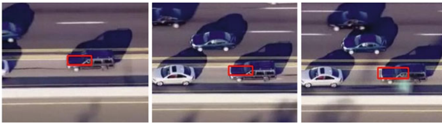
Fig. 11 Results of tracking by fusing Mean shift and Kalman. Frame1, 110, 171 (left to right) are shown
