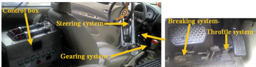
Fig. 5 The execution system
