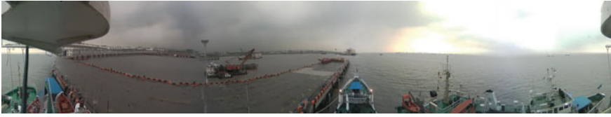
Fig. 5 This image shows the result of panorama stitching and has a resolution of 2556 \times 470 pixel. The camera system is mounted on the pole of a ship. The image also shows a color correction algorithm that has not been implemented in the GPU-accelerated code yet. In some areas, the blending is not perfect. This could be improved by a better calibration of the lens distortion.
