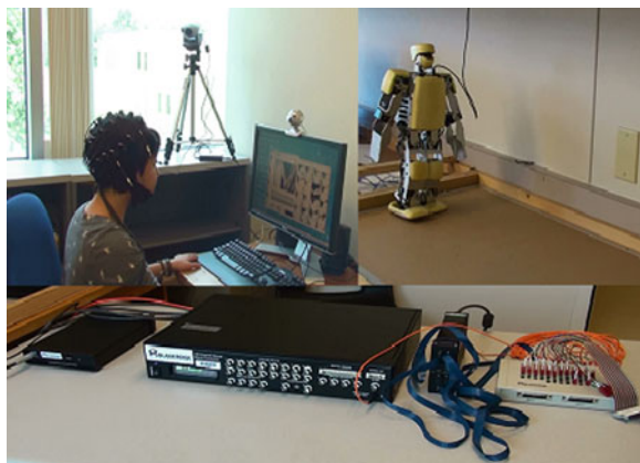
Fig. 1 Cerebot consists of a Cerebus TM data acquisition system and a humanoid robot
