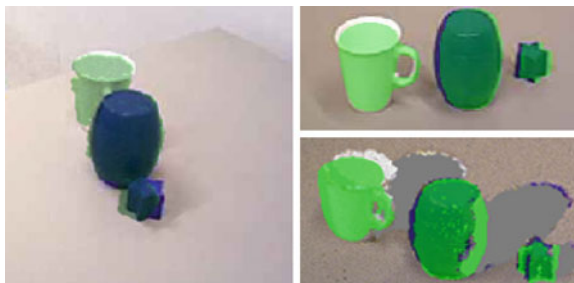
Fig. 7 The left image shows the partial occluded scene. The segmentation delivers an under segmented cluster. After the perspective change the recognition can be applied successfully. The right images show the visualization of a successful recognition in the image ( top ) and the point cloud ( down )
