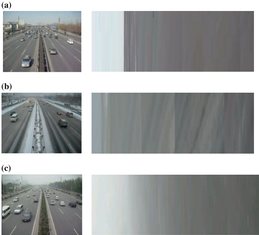
Fig. 2 Traffic scene and the corresponding extracted area which are enlarged. a original image and extraction result for sunny in scene I, b original image and extraction result for snowy in scene I, c original image and extraction result for fog in scene I
