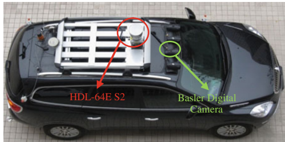
Fig. 4 Alignment of the HDL-64E S2 lidar and the Basler digital camera
