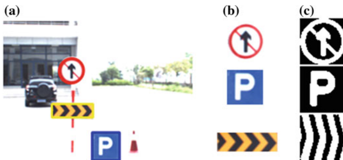
Fig. 6 Shape analysis and normalization. a Results of shape analysis and traffic signs labeling; b Extracted ROIs images; c ROIs normalization and binarization ( 51 \times 51 resolutions)
