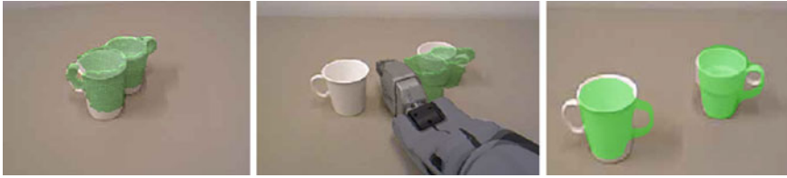
Fig. 8 The left image shows the under segmented scene, the feature detectors deliver no useful information. The recognition is not possible. The middle image visualizes the influence in the scene with the manipulator. After re-applying the segmentation and feature detectors the objects can be recognized
