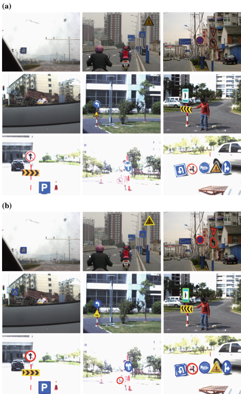
Fig. 8 Traffic signs detections. a Original images; b Detection results labeled with corresponding color and shape markers
