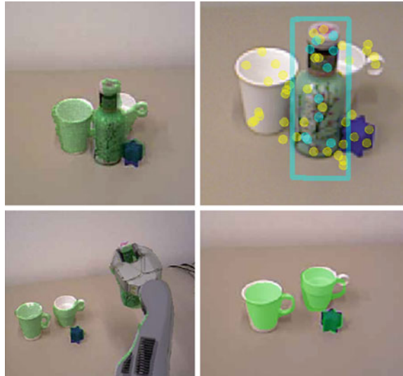
Fig. 6 The left upper image shows the under segmented cluster, the recognition of single objects is not possible. The SIFT/SURF detector recognized the bottle (bounding box in the right upper image). In the left lower image the manipulation with the PR2 is visualized. The robot grasps a bottle and removes it from the scene. After re-applying the segmentation and feature detection the rest of the objects can be recognized
