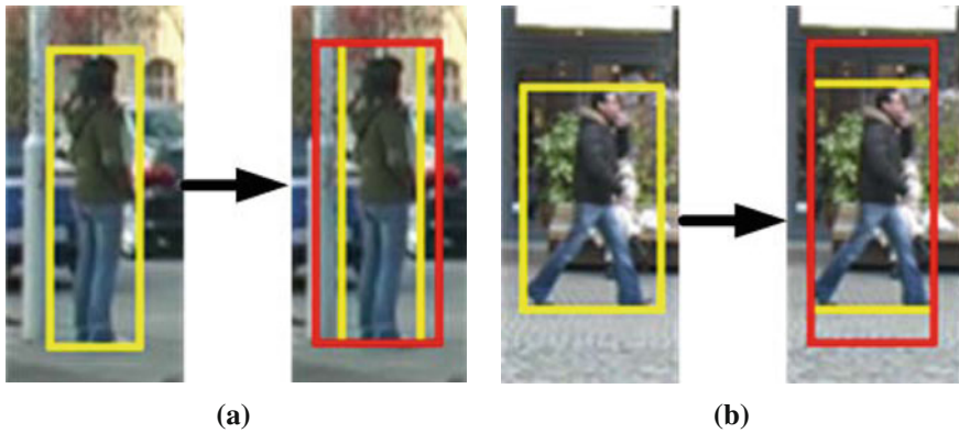
Fig. 3 The aspect preserving rescaling scheme. See text for details. a r_0 \geq r_i . b r_0 < r_i
