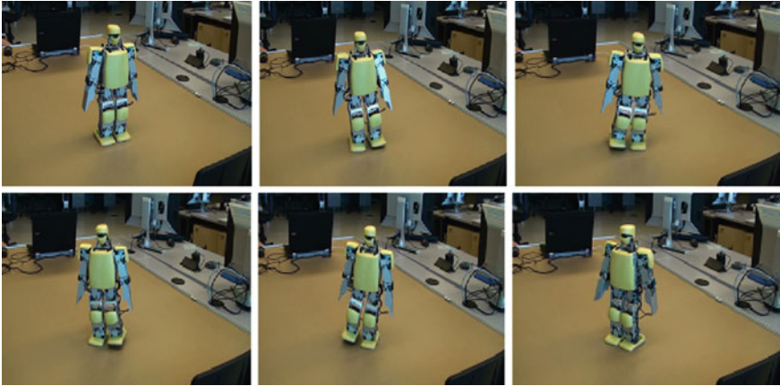
Fig. 8 Control of robot turning left with imagination
