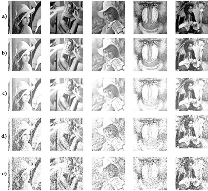
Fig. 4. Images of set-1, (a) original image. Altered images, erosive noise (b) 60%, (c) 100%; mixed noise (d) 30 %, (e) 40%.
