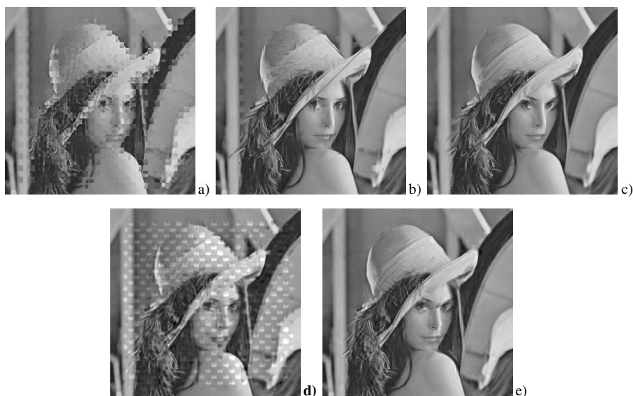
Fig. 3. Error distribution: checkerboard. Concealed image Intra of “Lena” with the: a) WAI, Y-PSNR=23.13dB; b) Directional Interpolation, Y-PSNR=25.86dB; c) Our method DI, Y-PSNR=28.44dB; d) FSE all 8 MB's, Y-PSNR=23.42dB; e) Our method FSE, Y-PSNR=28.34dB.
