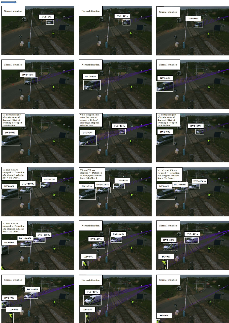
Fig. 11. Danger evaluation and recognition of potential dangerous situations. DV_i represents the danger related to the vehicle number i and DP represents the danger related to the pedestrian.
