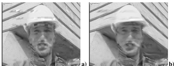
Fig. 6. Error distribution: bursty. Concealed image Intra of “Foreman” with the: a) FSE weighted 0.1, Y-PSNR=26.84dB; b) Our method FSE, Y-PSNR=27.25dB.
