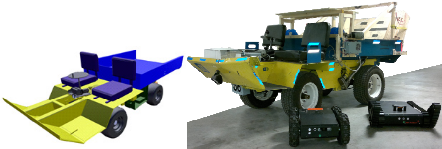
Fig. 6. Marsupial Robotic Team (MarRT). On the left, the CAD model of the carrier robot generated through inverse engineering for simulation and design of mechanical components. On the right, actual electrical vehicle instrumented through a CAN-based network controlled system and two of the search and rescue robots it can transport to a deployment point.
