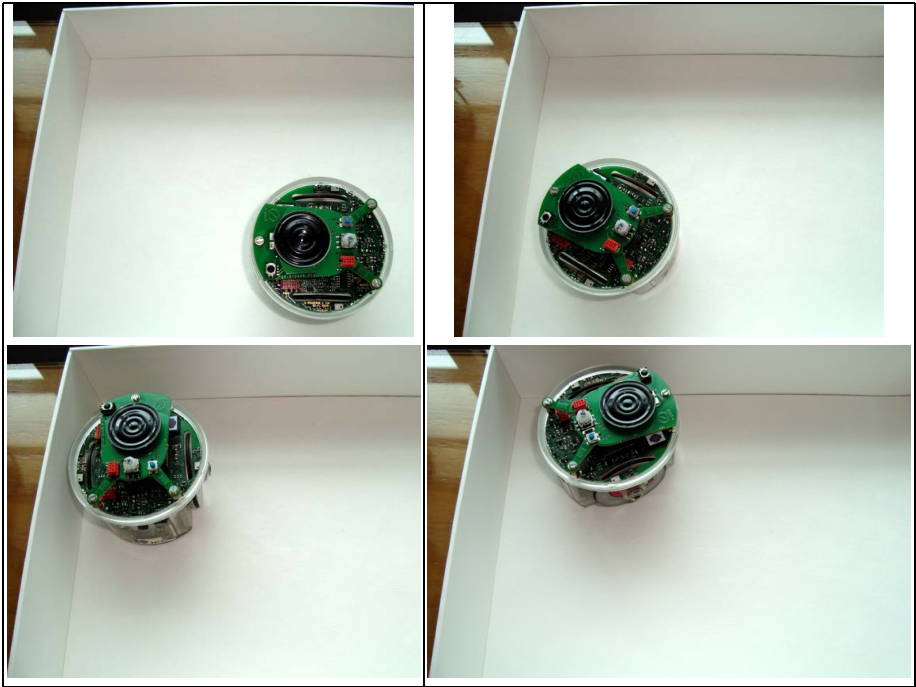
Fig. 5. Robot behavior in the real e-puck robot for the best individual of evolution using the DE/best/1/bin method. The robot starts searching for a wall, when a wall is found, the epuck follows the wall while avoids crashing into walls.
