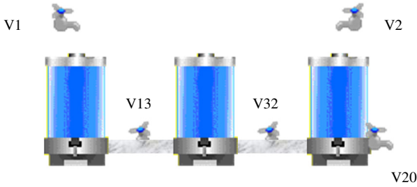
Fig. 2. Water control of 3 tanks
