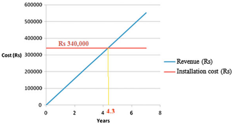
Fig. 36.1 Payback period for the installation of PV panel to produce 10 MW of electricity/year
