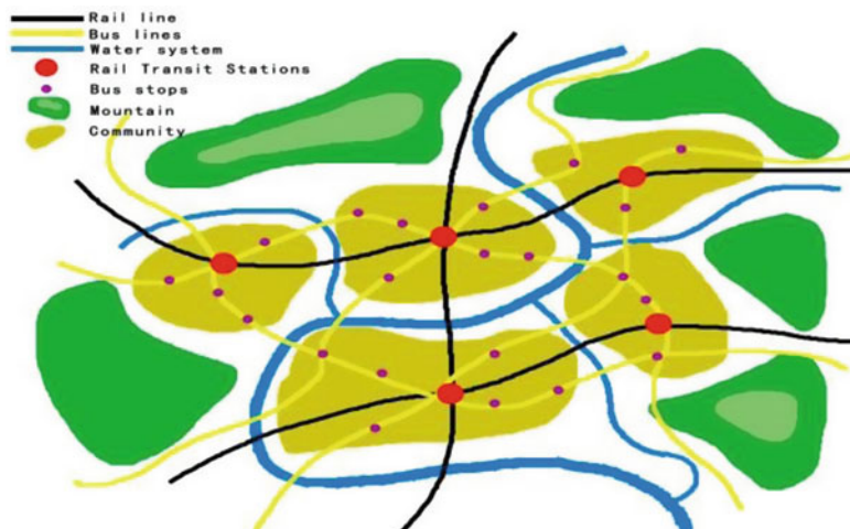
Fig. 11.5 Schematic diagram of park-ride and community divided way based on reach ability regional
