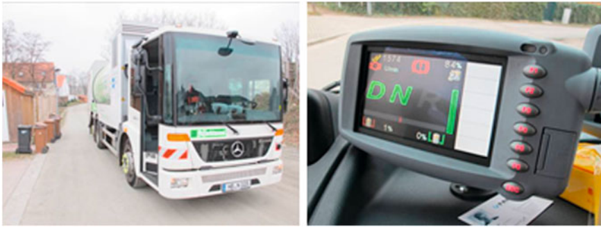
Fig. 5 Hybrid waste collecting truck in Bremen/cockpit display for electric components
