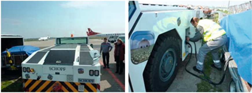
Fig. 4 Full battery electric pushback truck in test at Bremen airport (2010)
