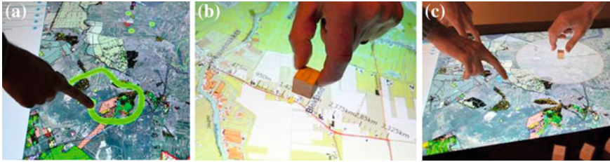
Fig. 2 Details of the user interaction: a sketching with a finger, b using a physical object to display a dynamic scale, c placing and rotating a small wooden block to define the center and size of a buffer/distance
