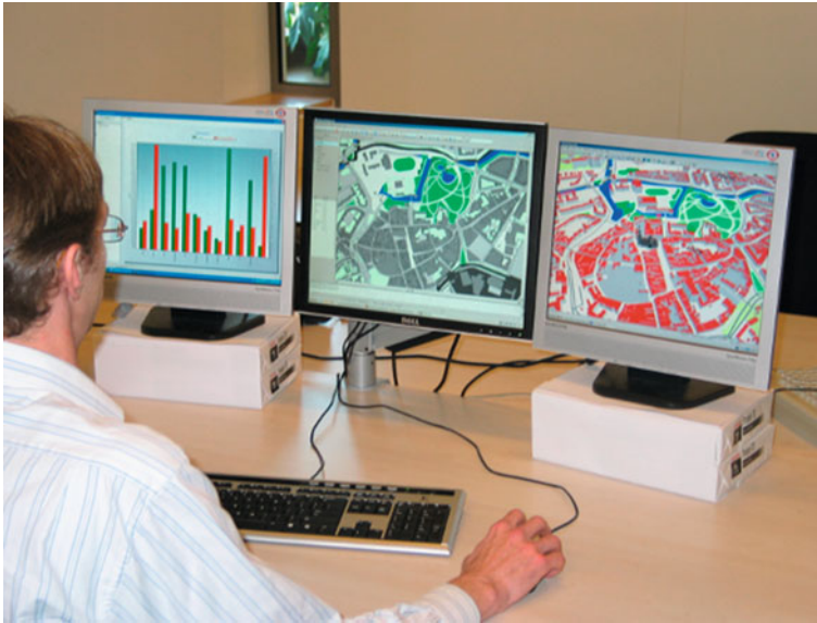
Fig. 3 Impact outputs of Urban Strategy . Left indicators in 1D, Centre 2D map which also has editing functions, and 3D visualization that can show model outputs (such as noise or air pollution contours)
