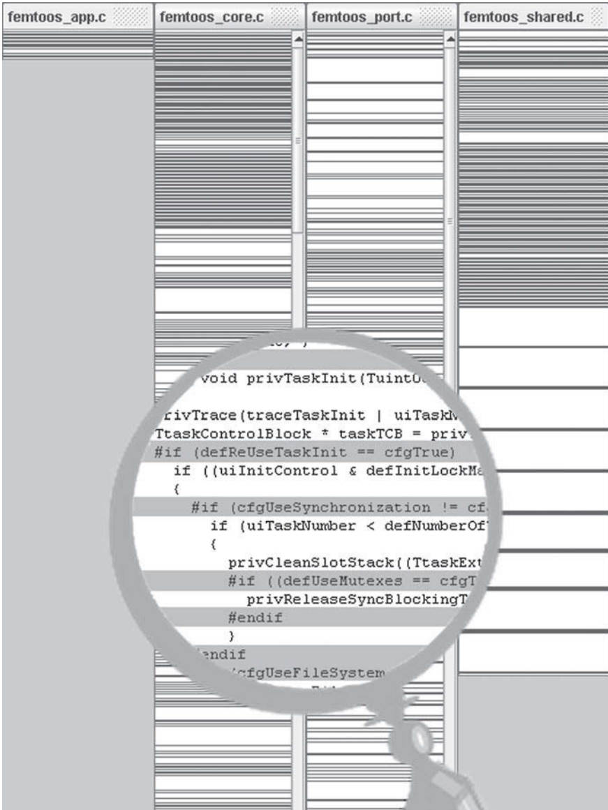
Fig. 5.17 Preprocessor directives in the code of Femto OS : highlighted lines represent preprocessor directives such as #ifdef , white lines represent the remaining C code, comment lines are not shown
