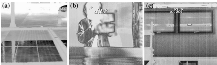
Fig. 5 Importance of reflective surfaces on thermographic measurements: a effect of reflectivity on the thermal image of a ceramic floor. b reflection of the operator on a metallic surface. c reflection of a light bulb in a window
