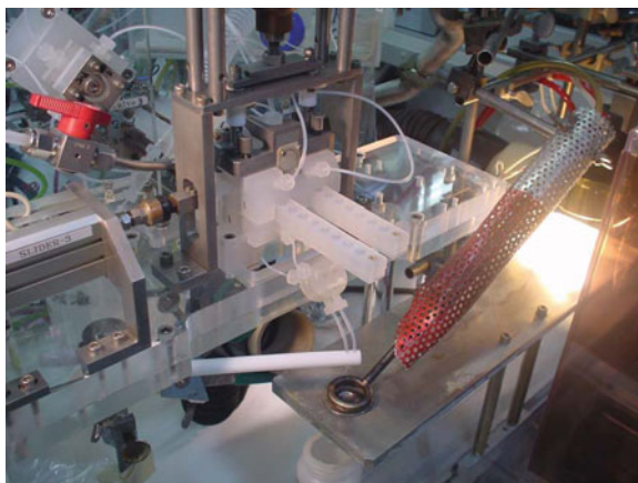
Fig. 13 Photograph of the chromatographic and sample collection part of AIDA
