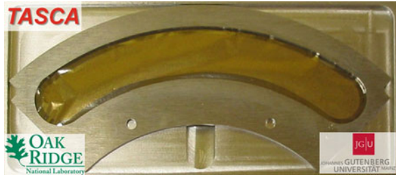
Fig. 2 Photograph of one segment of a rotating ^{249}\text{Bk} target on 5 \mu\text{m} Ti backing fabricated by molecular plating at Mainz University with material supplied by Oak Ridge National Laboratory. (photograph courtesy of Mainz University)
