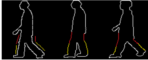
Fig. 7. Points to be taken for regression Red for thigh angle and yellow for calf
