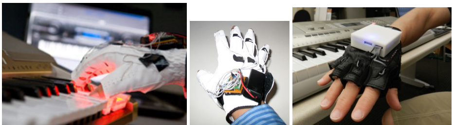
Fig. 3. Vibrating motors of Mobile Music Touch cue which fingers to play
