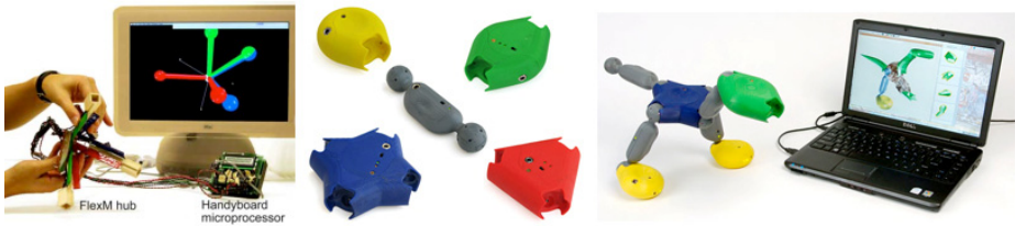
Fig. 2. FlexM is a computationally enhanced hub-and-strut construction toy. Posey is an interface of optocouples ball and socket joints and struts that can transmit wirelessly to different domain applications such as an online puppet show.
