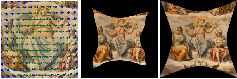
Fig. 1. Left: example image acquired by a central camera with high radial distortion, and superimposed the optical flows computed using two small camera rotations. Centre: undistortion obtained with the state-of-the-art method in [18]. Right: global undistortion obtained with our non-parametric linear method; its average global error is 2 pixels, from which only 0.5 pixels correspond to non-perspective distortion.
