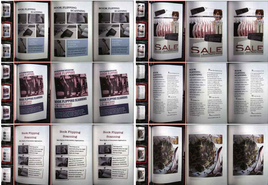
Fig. 10. Restored images of six example documents. In each example, the input image (left), image unwarped by TPS (center), and the image unwarped by the proposed method (right) are shown.
