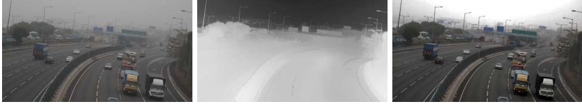
(a) Background-defogging when the foreground and background are nearly at the same depth.
