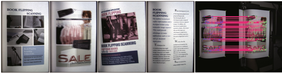
Fig. 9. Restored images after initial estimation and the example of feature point correspondence in the deformation reconstruction
