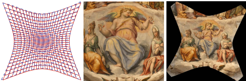
Fig. 2. Left: groundtruth sensor (red lines) and the estimated undistortion map (dashed blue lines). Centre: original image smoothed using the metric induced by this map. Right: mosaic performed with the Z rotational sequence of calibrated images.
