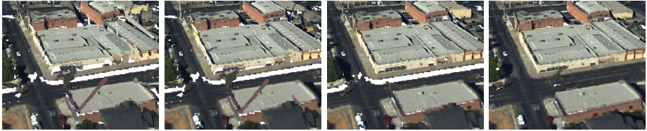
Fig. 2. Reconstruction results according to the iteration. From left to right , plane initialization, refinement, optimization, and after multiple refinement and optimization steps.
