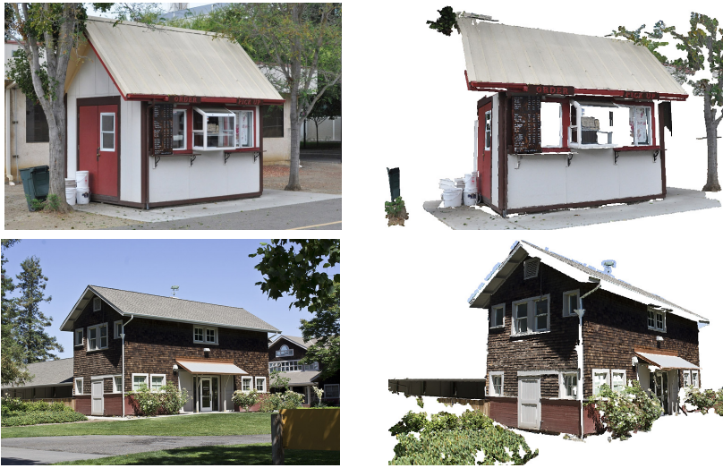
Fig. 7. Two outdoor scene reconstruction results. Each row shows one of the input images ( left ) and its reconstructed scene ( right ).
