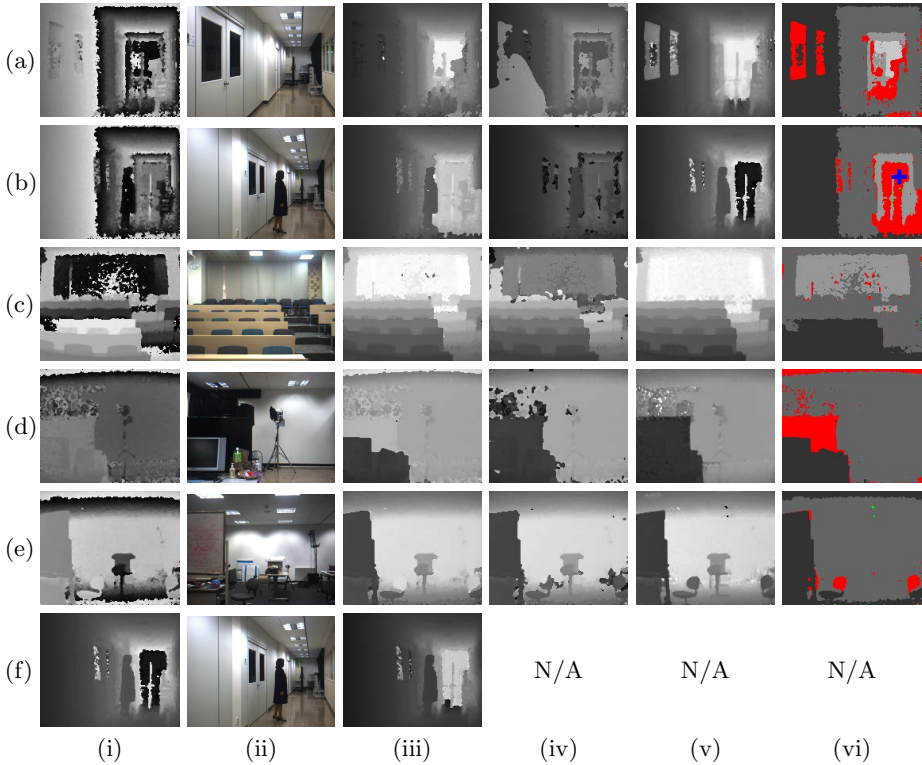
Fig. 4. Phase unwrapping results. (i) Input depth map. (ii) Left image. Unwrapped depth maps obtained by (iii) the proposed method and (iv) MFPU. (v) Ground-truth depth map. (vi) Estimated number of wrappings corresponding to (iii). The maximum intensity (255 in gray level) in (i) corresponds to 5m except the last row (15m). It corresponds to N \times 5\text{m} in the other depth maps in (iii–v), where N = 3 for (a),(b), N = 2 for (c),(d),(e), and N = 4 for (f). The gray level intensity in (vi) is linear with the number of wrappings ranging from 0 to 3. The red pixels are with erroneously estimated numbers of mods, while the green pixels are those discarded from the evaluation.
