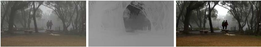
(b) Background-defogging when the depth between foreground and background is large.
