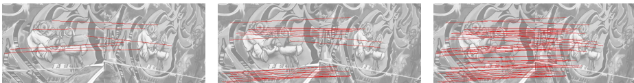
Fig. 3. Robust homography estimation. From left to right: RANSAC threshold (transfer error through homography) T = 0.5 pixels yields 6 points correspondences, threshold T = 2 pixels (i.e., default Bundler threshold) yields 19 points, and threshold T = 6.8 pixels yields 50 points as well as a better estimated homography. This last value was actually automatically computed with an a contrario technique, that statistically determines a confidence threshold (cf. Section 4).
