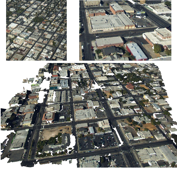
Fig. 9. Aerial urban scene reconstruction (Stockton, CA, USA). One of the input images ( left top ) and a reconstructed scene ( right top, bottom ).
