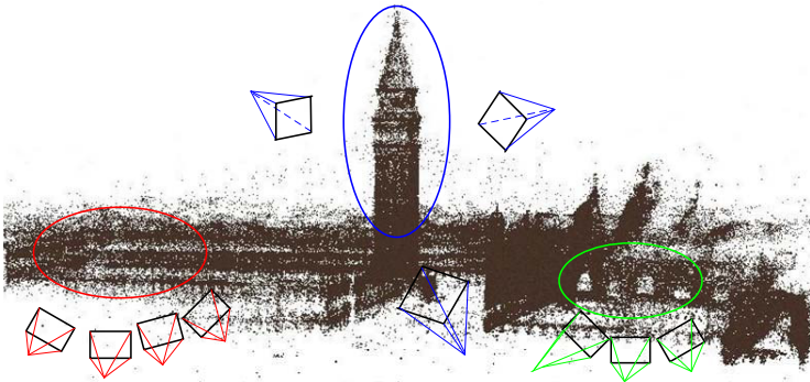
Fig. 1. Illustration of sparsity of BA. 3D points in blue ellipse are mainly reconstructed by cameras marked in blue, and these 3D points have fewer projections on images marked in red and green. Cameras marked in red and green photograph different parts of the scene, and thus no 3D points to connect images in red and green together. Remarks: 1) The Venice model with 1778 cameras is optimized by our VPBA algorithm, and this initial 3D model is released by Agarwal et al [15]. 2) Only schematic positions of a few cameras are illustrated.
