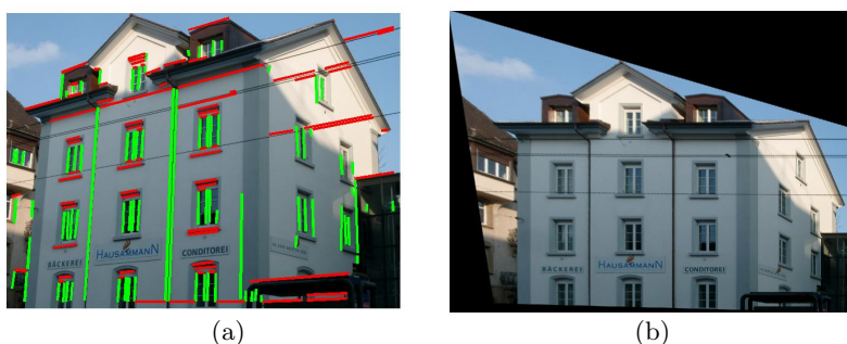
Fig. 2. Image rectification. (a) The original image with detected line segments, that are consistent with the two vanishing points. (b) Fronto-parallel rectified image.
