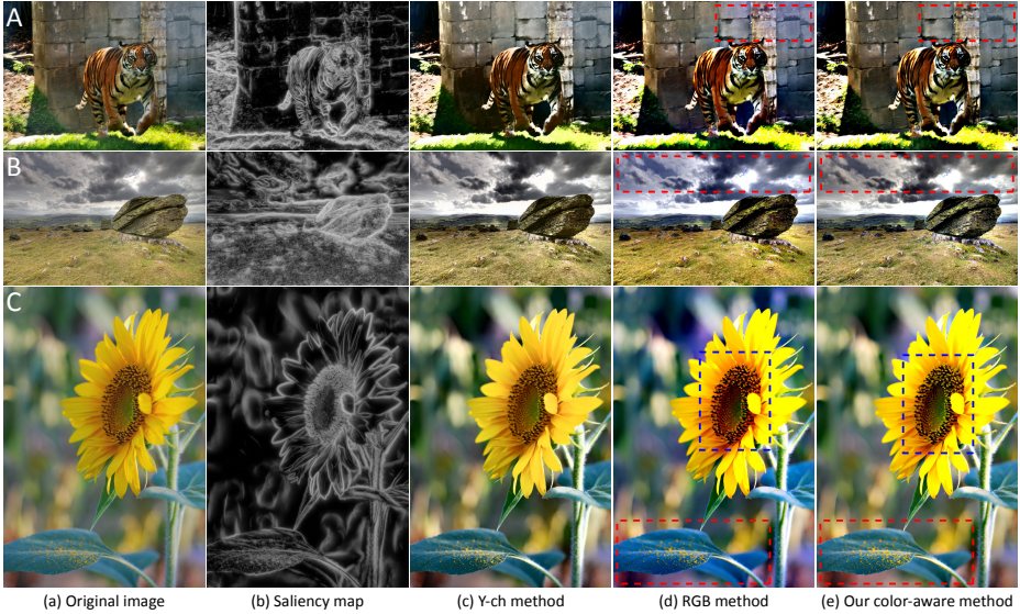
Fig. 7. Examples of saliency sharpening: (a) input RGB image; (b) saliency map of the input image; (c) result using L_2 regularization over the Y channel only; (d) result using L_2 regularization over R/G/B channels; (e) our color-aware regularization result. Regions with color-shifting problem have been highlighted in red and blue dashed boxes.
