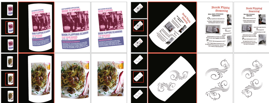
Fig. 5. The synthesized input images and the restored images. Four example results are shown. In each example, the input image and the enlarged image (left), image unwarped by TPS (center), and image unwarped by the proposed method (right) are shown.
