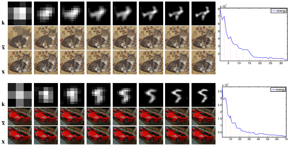
Fig. 4. We show for the first two examples from Fig. 3 a few snapshots of k , \bar{x} and x as estimated during the course of our deconvolution algorithm. We also show corresponding energy plots (where red dashed lines indicate a change in resolution).
