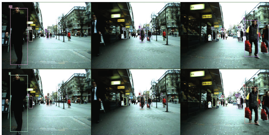
Fig. 9. The top row shows the result of running the DP (with NMS) tracker of [6] on part of the ETHMS sequence. The bottom row shows our result. Our algorithm does a better job at maintaining ID labels over time.
