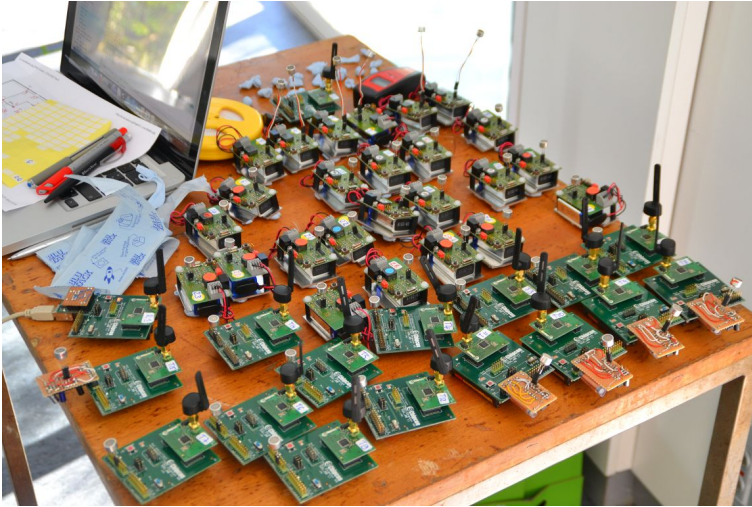
Fig. 7. Hardware used for the test run: Visible are 25 receiver nodes (table left side), 15 calibration nodes (table right side), 5 of them equipped with ultrasound booster amplifiers, and a notebook acting as iLoc server.
