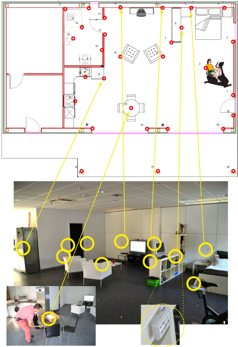
Fig. 8. Installation of 30 RFID tags in the Living Lab of the Polytechnic University of Madrid, Spain
