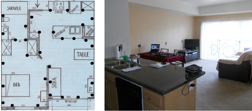
Fig. 9. On the left, the blueprint of the single floor, one bedroom apartment in which the RTI system has been deployed for over three months. The black dots represent the position of the 33 RF sensors. On the right, an image of the apartment.
