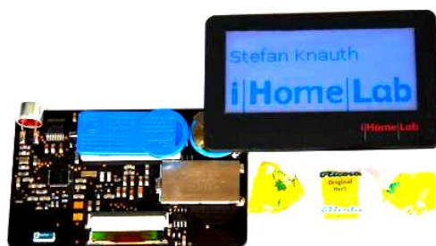
Fig. 3. Name badge with IEEE802.15.4 radio transceiver, ultrasound transmitter and LCD
