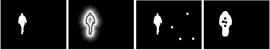
Fig. 4. Examples of computation of the D-Score. From Left to Right: a ground-truth image; cost map based on a DT; example of long ranges errors, leading to a D-Score of 0.003; omissions with medium range errors, with D-Score: 0.058
