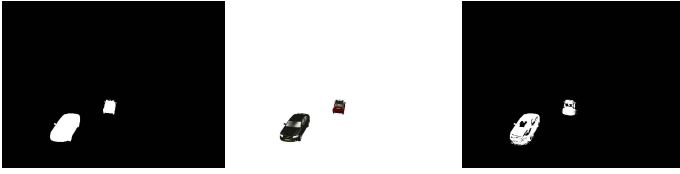
Fig. 3. To compute the SSIM, we need the intensities of pixels, in the ground truth sequence G (Left), and in the sequence computed by a BSA (Right)
