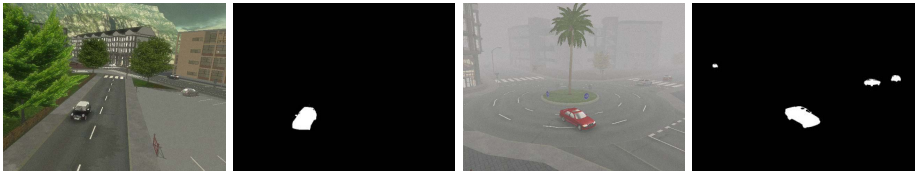
Fig. 1. Examples of synthetic videos and their associated ground truth in our dataset. Left: scene 1, configuration 3, use-case 1 (learning phase). Right: scene 2, configuration 4, use-case 2 (evaluation phase)
