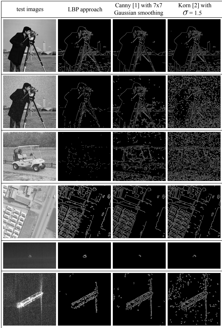
Fig. 7. Examples for real data processing: original images and edge detection using LBPs, Canny, and Korn (from left to right column)
