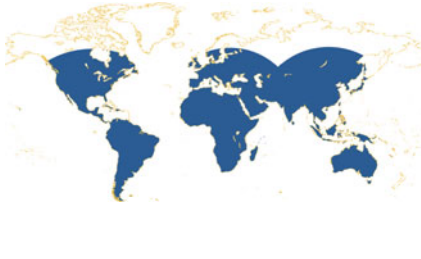
Fig. 25.1 Trimble CenterPoint RTX L-Band coverage using six geostationary satellites
