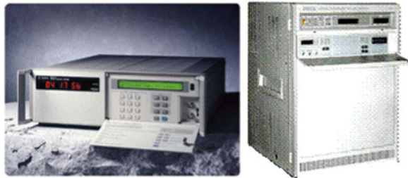
Fig. 43.1 Industrial Cs tube clock ( left ) and H-maser clock ( right ) with the stabilities respectively 10^{-14} and 10^{-15} in frequency or correspondingly 1 and 0.1 ns in time in one day
