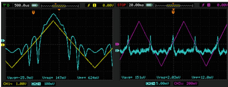
Fig. 31.4 Typical optical absorption signal (left, blue) and CPT resonances (right, blue) of microfabricated cells
