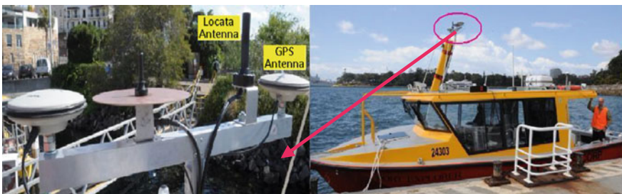
Fig. 54.3 Test vessel and installed Locata/GPS antennas
