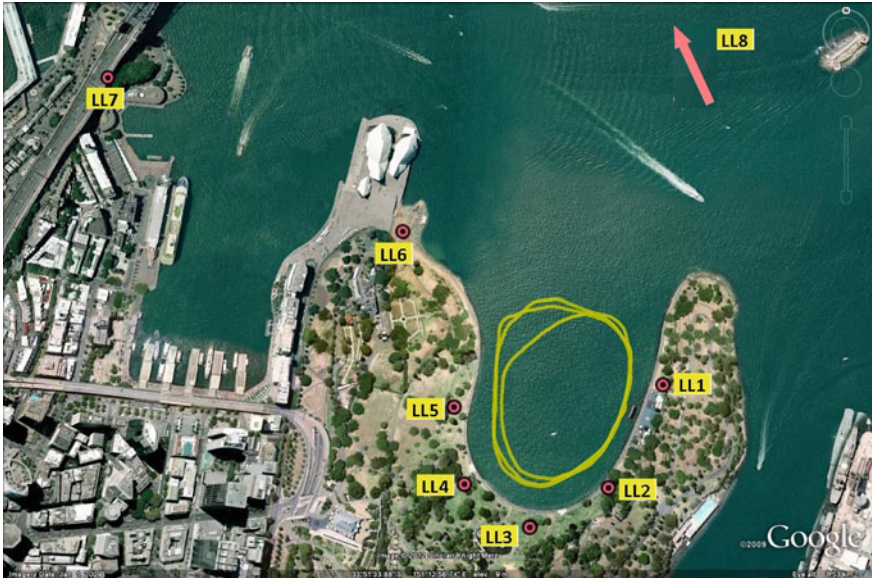
Fig. 54.2 LocataNet configuration and rover trajectory
