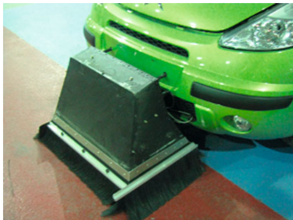
Fig. 2 Black metal box of the visual system
