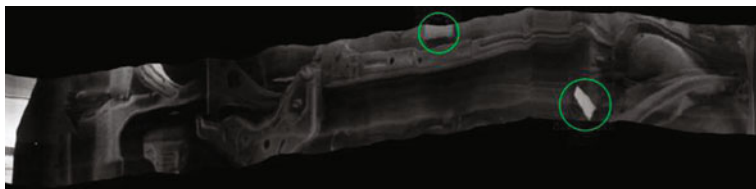
Fig. 4 Section of a scanned undercarriage which includes two ( circled ) simulated IEDs
