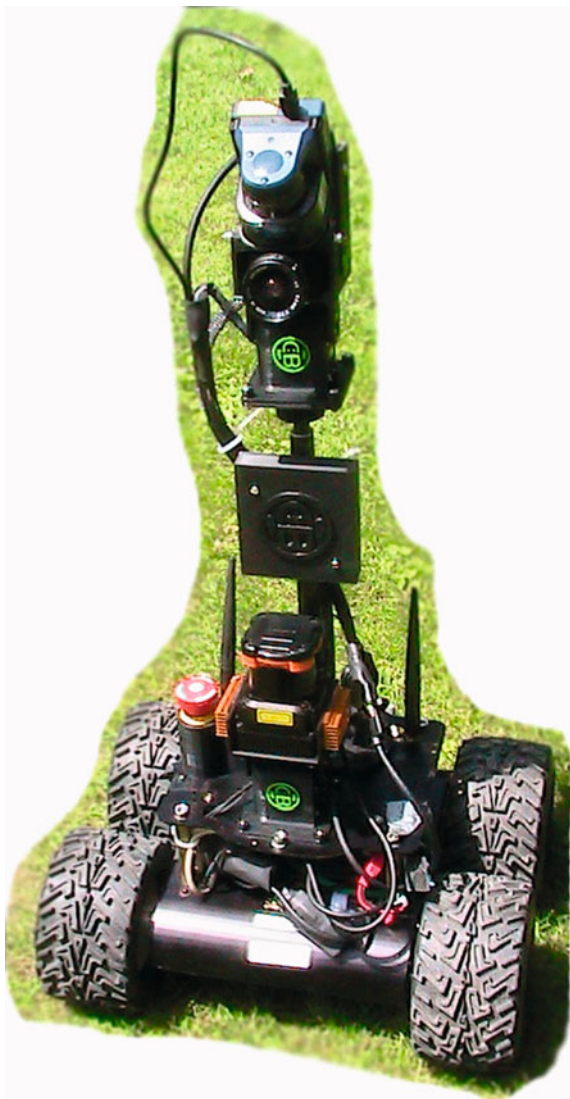
Fig. 1 Platform used: the WiFiBot
