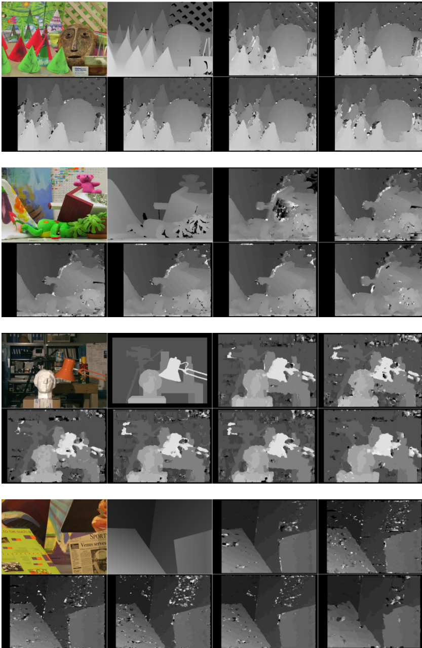
Fig. 3. Comparison of the disparity map for the Middlebury dataset (Cones, Teddy, Tsukuba, Venus). From left to right (First row): Left Stereo image and its local ground truth disparity map, SAD, Census, (Second row): Census Sparse, Rank, Rank Sparse, Proposed method.
