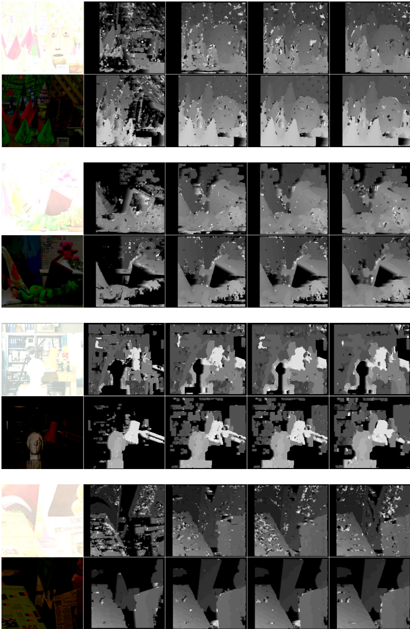
Fig. 4. Comparison of disparity map in different brightness and exposure for Middlebury dataset (Cones, Teddy, Tsukuba, Venus). From left to right SAD, Census Sparse, Rank, Proposed method.
