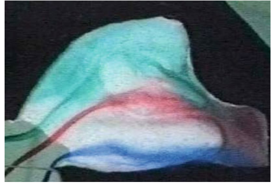
Fig. 20.8 Flow-experimental presentation of inspiratory airflow in a nose model without a vestibulum. The concave curved surface of the internal nasal orifice causes divergence of the flow paths in the cavum
