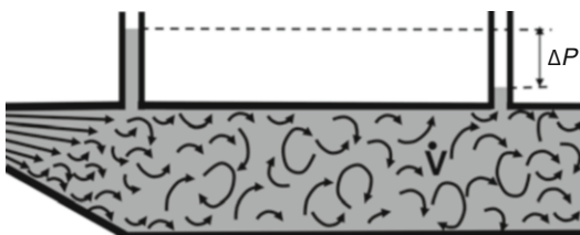
Fig. 20.4 Flow paths in a flow channel with turbulent flow ( \Delta P =friction-related pressure loss, \vec{V} = flow velocity)
