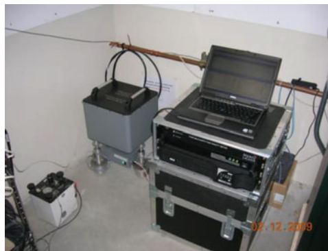
Fig. 1 The spring gravimeter gPhone#032 on its tilt controlled tripod and electronics
