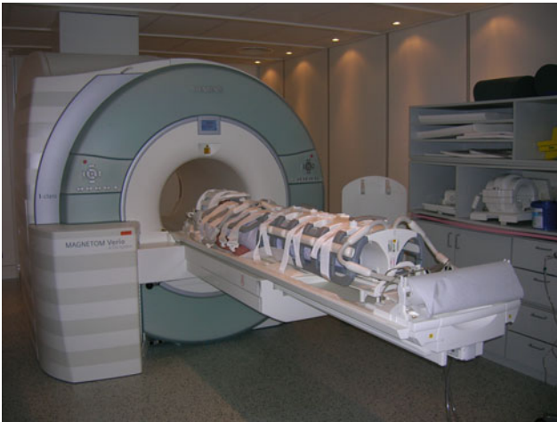
Fig. 8 Whole-body MRI. To obtain whole body MRI images, the entire body is covered in coils (image courtesy of Prof. Dr. M. A. Weber, Heidelberg)
